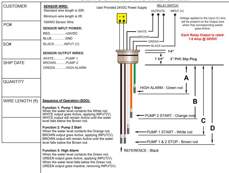
System Dynamics, Inc. P.O. Box 12544 Scottsdale, Arizona 85260 Toll Free: 866-243-2505 sales@waterlevelcontrols.com www.waterlevelcontrols.com All rods are 304 stainless steel with 1/4-20 threaded ends. Sensor rods can be extended using an Extension Rod kit accessory. Sensor rods & wires are Intrinsically safe with circuit limited signals.
