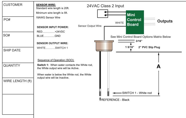
System Dynamics, Inc. P.O. Box 12544 Scottsdale, Arizona 85260 Toll Free: 866-243-2505 sales@waterlevelcontrols.com www.waterlevelcontrols.com All rods are 304 stainless steel with 1/4-20 threaded ends. Sensor rods can be extended using an Extension Rod kit accessory. Sensor rods & wires are Intrinsically safe with circuit limited signals.
