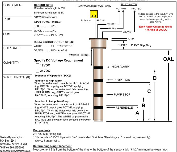
The Over All Length is measured from the bottom of the sensor cup to the bottom of the sensor stick.
